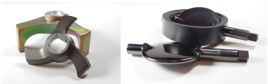
Fig. 2: DC99® and STech® coated parts for the food industry; request: non-stick, reduced wear and friction, food-safe (left) and DC99® DLC layer on a valve for the chemical industry; demand: anti-fouling properties, low friction coefficient and wear protection (right)
