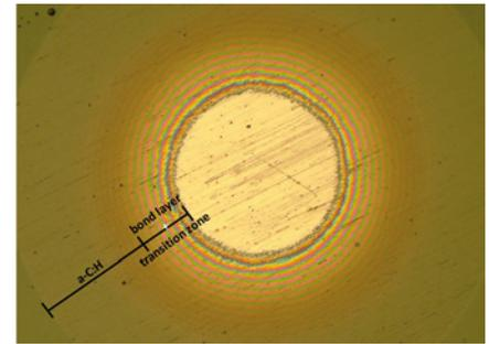
Fig. 1: DC99® DLC layer: dense, compact and amorphous with a smooth as deposited coating surface. To achieve such a morphology and thus the corresponding properties a surface finish  $R_a < 0.1 \mu\text{m}$  of the to be coated component is demanded; the ball crater (right hand image) illustrates the coating design of the DC99® DLC layer
